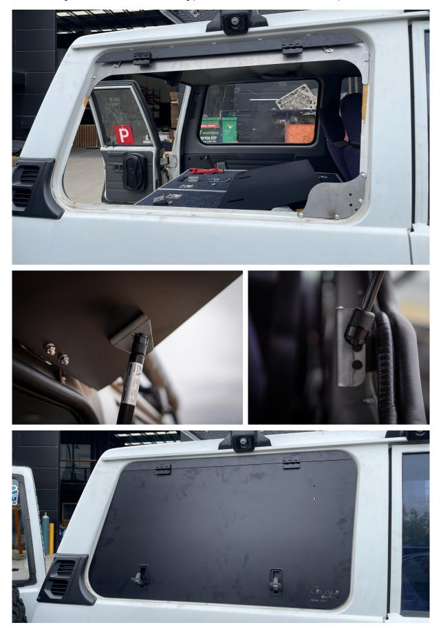
**STEP 10**: Fit the gas strut and adjust the locks.
