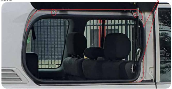
Grab your rubber pinch weld and fit it to the window opening as show above. Cut it to length, then remove it, apply mastic the entire way around where the pinchweld mates to the window opening (DO NOT SKIP THIS STEP)
