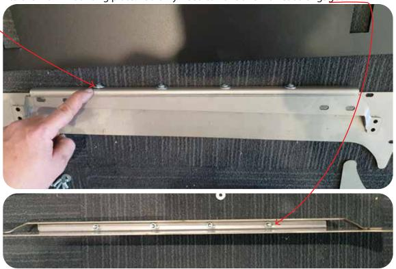
Loosely install the hinges through the "cover top" into the hinge mounting plate using the m6 washers and nuts.
