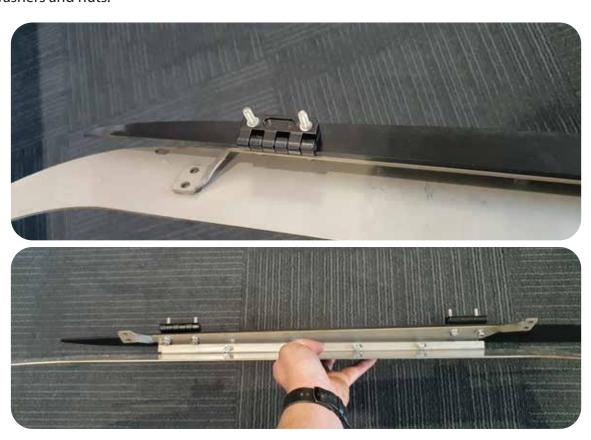
Install the m5 bolts, washers and nuts through the holes pointed to below. Hand tighten them all the way. Not so tight you can't adjust them though.
