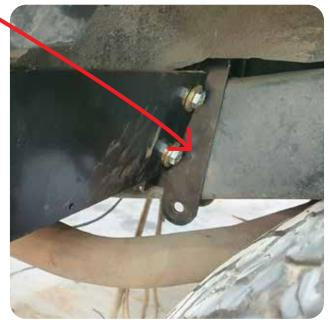
Install the chassis clamps as show above (top right) You can also put the clamp on from underneath depending on your exhaust/long range tank,
