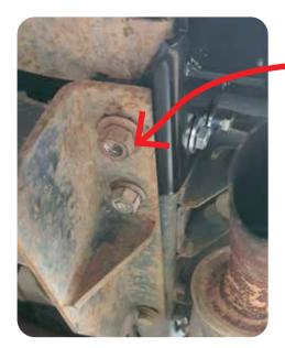
Loctite and loosely install the m10x35 with load rated washers into the nut plates on both sides of the chassis. Loosely install the 4x m12x50 1.25 bolts with large gold washers into the captive nuts. If you have no captive nuts on the drivers side you will need to reuse the tow bar nut plate or drop the bolts down from the top and install the nut with large washer.
