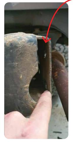
Insert the nut plates into the chassis so the nuts line up with the holes further in the chassis (Don't bolt them up yet)
