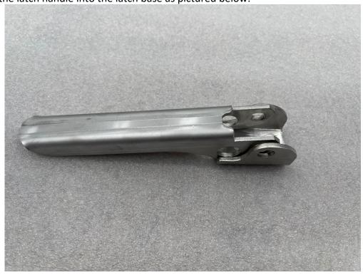
STEP 2: Install the 2x small pins with circlip grooves through the latch handle and the latch base. Please ensure the pins go from the top down so that the circlip is fitted on the bottom of both pins, this means that the left and right latch handles will have pins installed in opposite directions. Please see pins intalled below:
