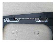
19. Flip the window and rest it on the hinges on a smooth surface that will not scratch the hinges or the window mounting panel and then assemble the hinges on the stainless-steel standoff with the supplied nuts and washers, leave the nuts loose so the window panel can slide.
