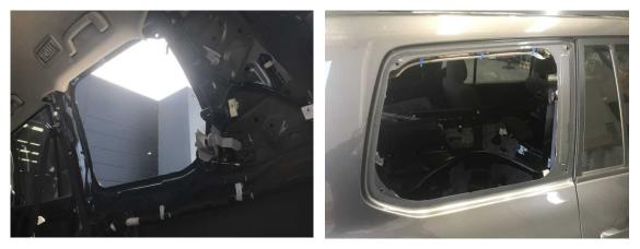
10. Once the window is removed there will be adhesive on the body, as seen in the right hand photo above, this can be left on the car and new Sikaflex can be applied over the top, however depending on the final alignment of the window some of the original adhesive may be slightly visible. To remove the remaining adhesive a suitable solvent, a plastic scraping tool (a trim removal tool can be used), together with some elbow grease is required. A cleaned passenger window is shown below.
