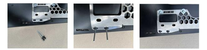
16. Next the lower gas strut mount is installed on the window mounting panel, take the components shown below and fix the bracket in the orientation shown.
