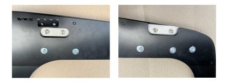
20. Next fix the tail of the fixed window panel to the window mounting panel using the third supplied rivet. Take care and consider using masking tape to protect the face of the painted rivet as scratches from the rivet gun will be visible.
