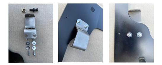
17. Now bend out the other tab on the window mounting panel by hand approximately 10°, this will be used to fix the tail of the fixed window panel.
