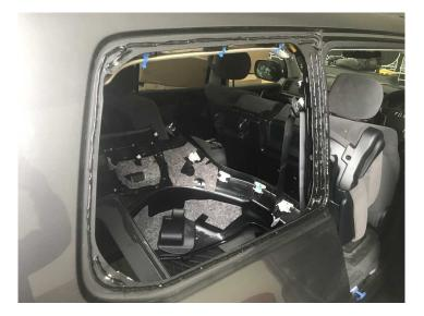
33. On the rear of the window apply Sickaflex to the edges marked below, in the install of the window the seal from this edge must be checked to avoid leaks as it is close to the edge of the vehicle body lip.
