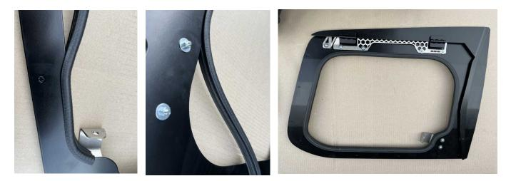
24. Next using the supplied nuts and washers attach the opening window panel to the hinges as shown below, again keep the nuts loose so the opening window panel can move slightly for adjustment
