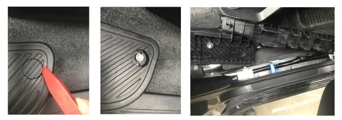
6. Now pop off the main side trim panel and then the rear upper white panel as shown below. On the passenger side the main panel has a wiring loom attached to it that must be unclipped. When fitting the drivers side window the antenna connection will need to be unclipped from the window.
