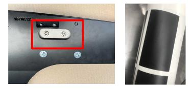
30. 'Dry fit' the window on the vehicle and check appearance, use the adjustment in the hinges if required. Then use an assistant to hold the window to the vehicle in the correct position and mark the pre punched holes on the vehicle body then drill out the holes in the vehicle body to suit the fastener you are using ( these fasteners have not been supplied).
